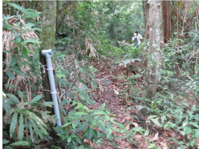
FIGURE 2. PVC pipe trap tied up on the tree trunk
